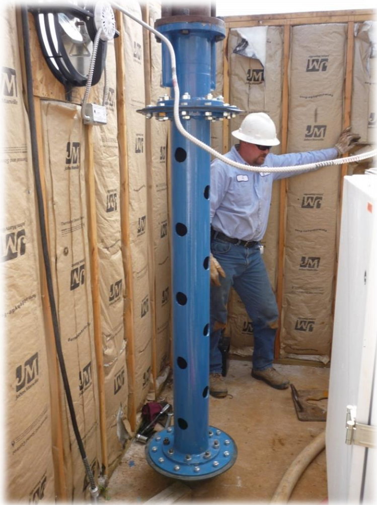
Double surge block / airlift development tool.
