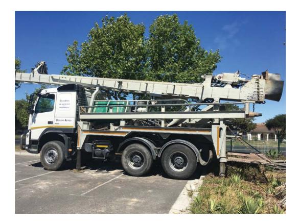
Figure 8: Down-the-hole hammer (DTH) rotary drilling rig
