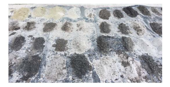
Figure 9: Drilling cuttings laid out at 1 m intervals
