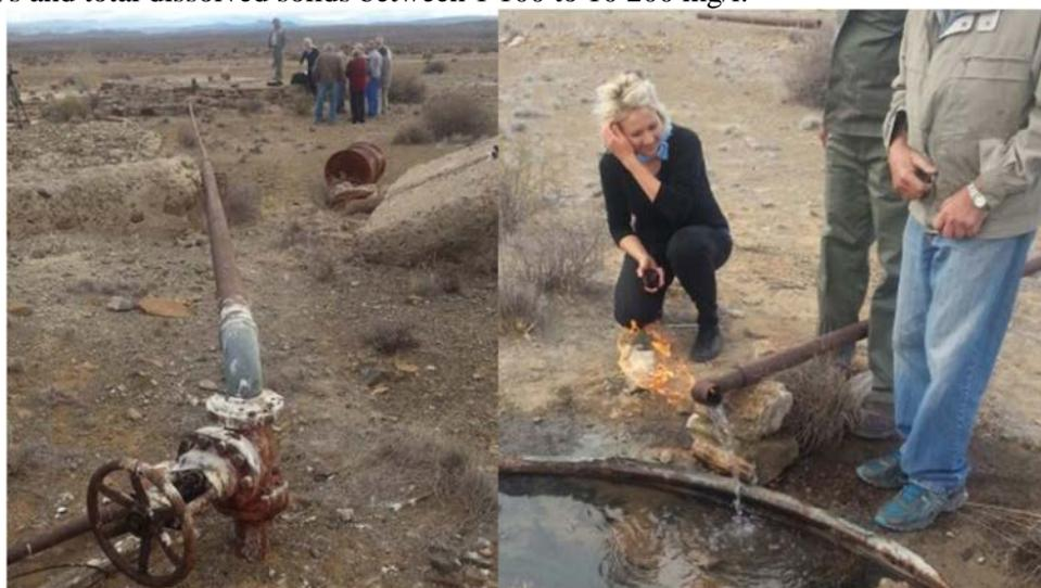
Fig. 3 Tap on artesian borehole SA 1/66 (left) and warm water containing methane flowing from it after tap was opened. Total dissolved solids = 8 100 mg/l
